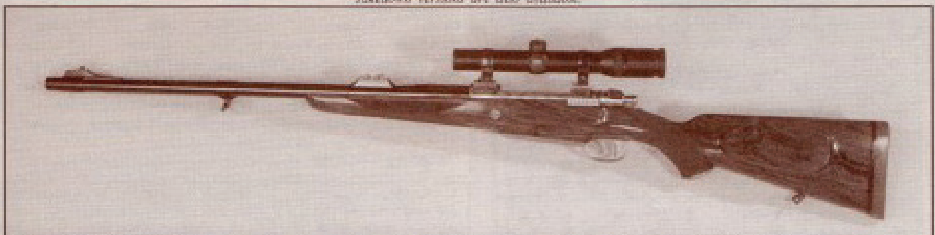
Jeffery with classic lines built by Reimer Johannsen. Quick-detachable scope mounts integral with double square bridges of the receiver allow use with a scope or iron sights.
